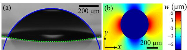
FIG. 2. (a) Optical side view taken from the  $x$  direction. The solid curve is a circular fit to the liquid-air interface, and the dashed curve is a parabolic fit to the bulge. (b) Optical profilometry scan taken from above the droplet depicting the  $z$  displacement  $w$  of the film surrounding the wetting region (dark elliptical area).
